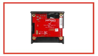
**Step 5** - Place the Amp within the top part of the case as shown in the picture. Make sure that the side panel is sliding within the plastic guides of the case.
