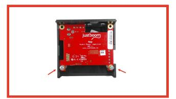
**Step 6** - Use the two metal screws to fix the part sitting on the white spacers glued to the enclosure.
