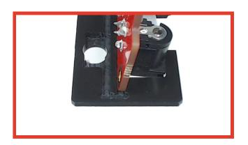
**Step 4** - Place the board onto one the side panel with two grooves so that it slots in the on the right as shown in the picture.
