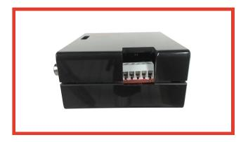
**Step 9** - Fit the bottom part of the case. The small indentation on it should be visible when looking at the case with the RCAs on the left and the Digital inputs on the right.
