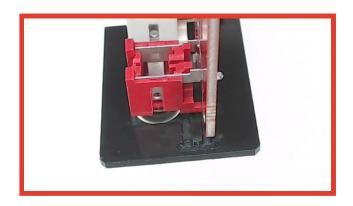
**Step 4** - Place the board onto one of the side panels so that it slots in the grooves as shown in the picture.
