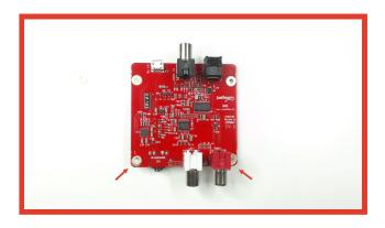
**Step 2** - Place the small plastic spacers on top of the DAC as shown here.
