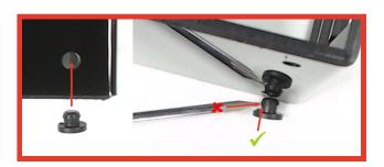
Step 3 - To install the rubber feet on the bottom part of the case you will either have to push and twist them through one of the 4 the holes or help yourself with a small screwdriver to tuck in the top part of the feet within hole as shown below. Be careful not to cut through the feet and rather than using the tip of the screwdriver use the flat surface to push the head of rubber foot in.
