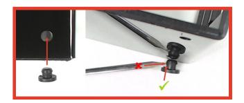
Step 5 - To install the rubber feet on the bottom part of the case you will either have to push and twist them through one of the 4 the holes or help yourself with a small screwdriver to tuck in the top part of the feet within hole as shown below. Be careful not to cut through the feet and rather than using the tip of the screwdriver use the flat surface to push the head of rubber foot in.
