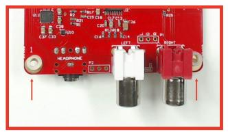
Remember that only two of the spacers are to be used and they will have to be positioned on the side of the RCA connectors.
