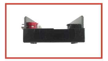
Step 6 - Place the board and the side panels in the bottom part of the case by making sure that the side panels are sliding within the plastic guides of the case. The small indentation of the bottom part of the case should be visible when looking at the case with the RCAs on the left and the Digital inputs on the right.
