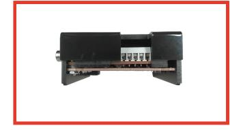
**Step 8** - Place the board and the side panels in the top part of the case by making sure that the side panels are sliding within the plastic guides of the case. The big opening of the top part of the case should be visible
