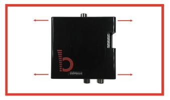
**Step 10** - As for when opening the case at the beginning, pull slightly the two sides of the bottom part of the case so that the plastic teeth can more easily slide in and hook on to the top part.
