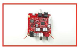
**Step 3** - Align the JustBoom Amp on the DAC as shown here and put the two cards on a side.
